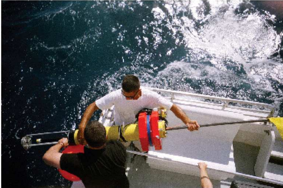
Photo shows AGS sensor deployment at the Eglin Air Force Base Joint Offshore Test and Training Area during a November 2005 operation. This particular sensor was equipped with an additional hydrophone and external digital recorder (note the small yellow Pelican case on the floatation collar, adjacent to the passive GPS antenna). This equipment was added to prove the concept of bottom impact detection.
