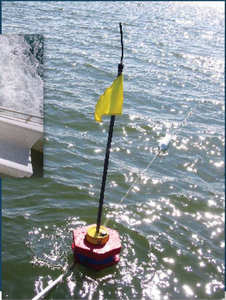
At left, a Joint Air to Surface Standoff Missile (JASSM) is seen just prior to impacting one of the Eglin Air Force Base Joint Offshore Test and Training Area floating targets. This particular test was conducted during a severe thunderstorm with seas estimated at seven to eight feet. Above and right, the deployment of TARGT hardware.
